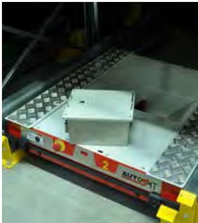
Longlife lithium battery removed for recharging
